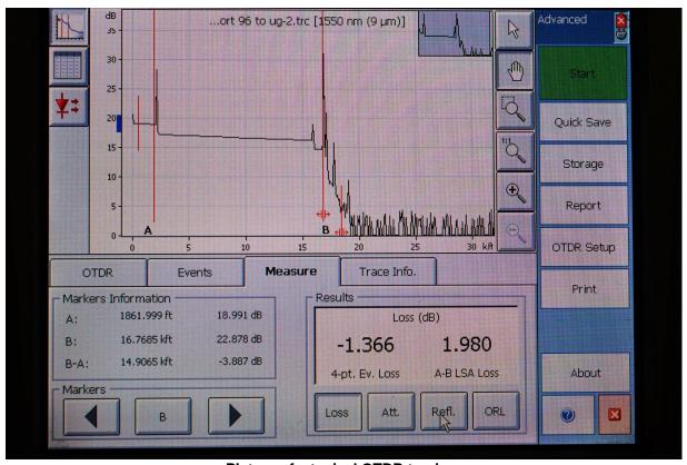
Picture of a typical OTDR tracing.
