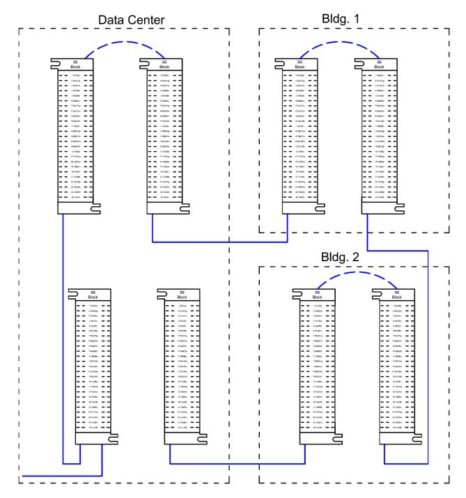
Physical Ring/Logical Star - A Copper cable is shown dropping off at each facility.
