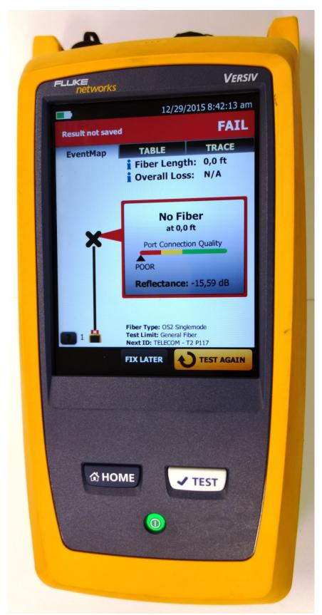
An Optical Time Domain Reflectometer is required to troubleshoot fibers.
