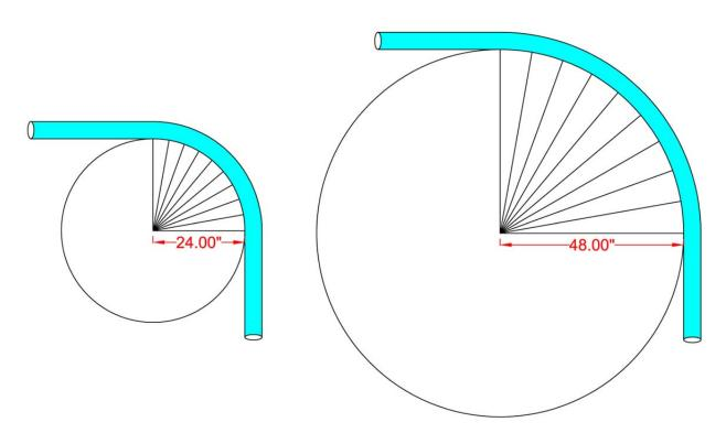
Bend radii requirements for fiber and copper cables.
