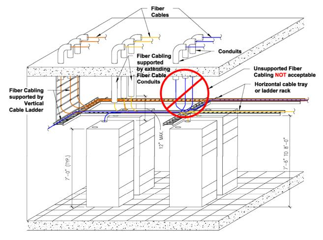
Vertical cable tray supports cables to the horizontal cable tray when conduits do not reach.
