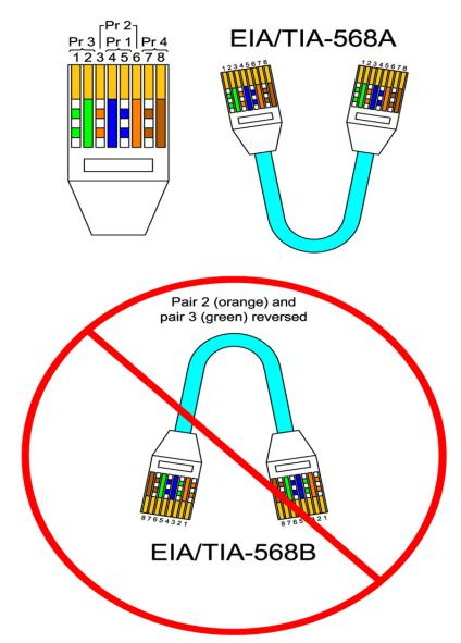
CAT 6/6A cable shall follow the EIA/TIA-568A wiring standard.
