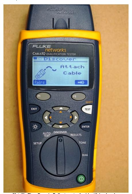
Metallic Time Domain Reflectometer for identifying breaks.
