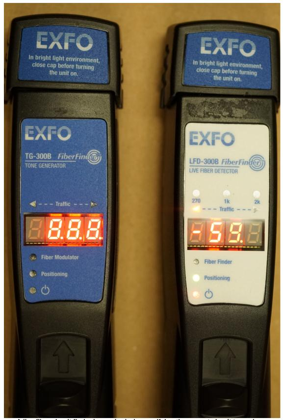
A live fiber circuit finder is required when verifying the correct circuit to work on.
