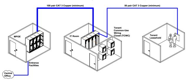
Backbone inside plant CAT 3 copper cables are extended from MPOE to IT Room to TCWC.
