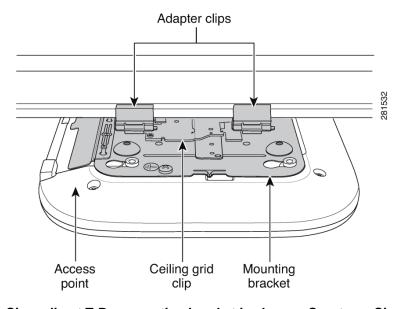
A Cisco direct T-Bar mounting bracket is shown. Courtesy: Cisco.
