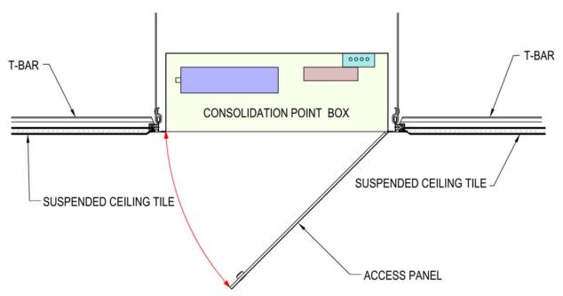
A sample Consolidation Point enclosure is shown attached to a suspended ceiling - side view.
