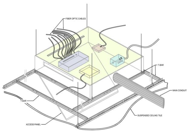
A sample Consolidation Point enclosure is shown attached to a suspended ceiling - iso view.
