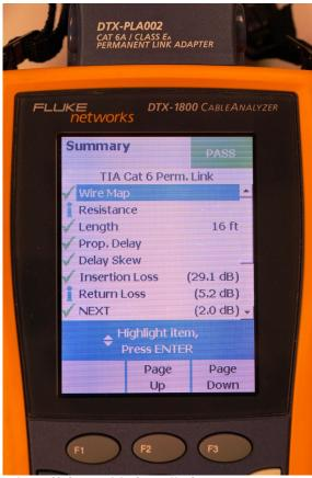
CAT 6/6A tester required for testing and certifying cable installations.
