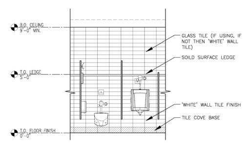
Figure 1.09.2B WALL FINISH AT URINALS AND WATER CLOSETS
