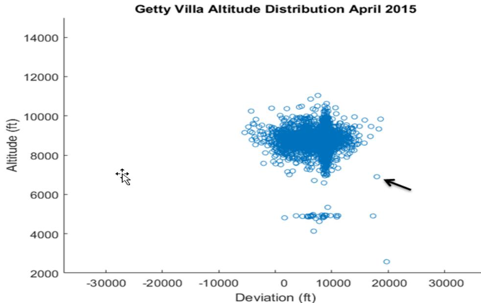
The x-y scatter plot seen in Figure 26 can be used to represent all of the gate crossings over a period of time – for example one day, one month, or one year. However, this visualization of gate crossing points is less helpful when analyzing a large number of crossings due to overlap.
