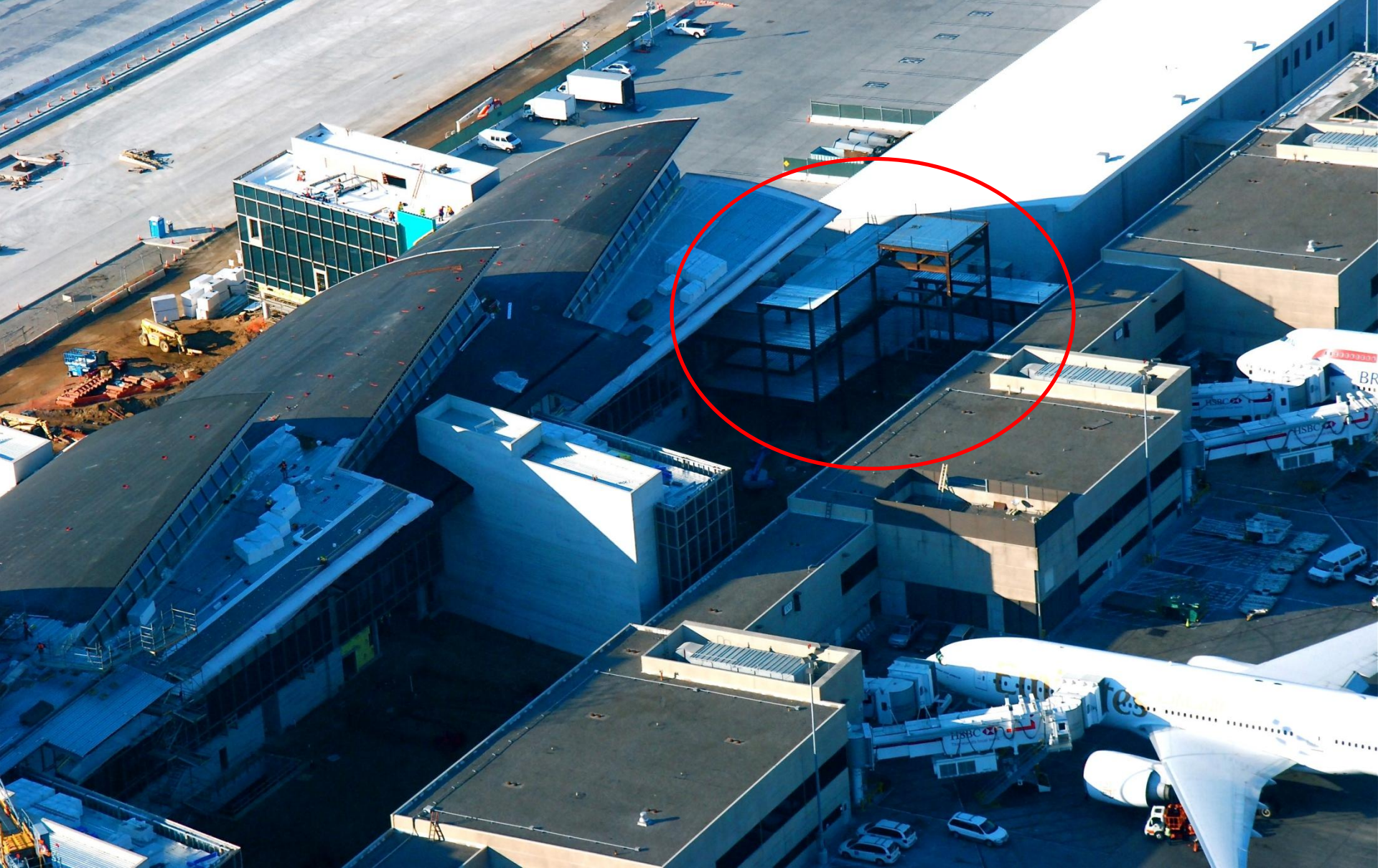
Aerial view of the temporary connector between the old and new concourses (circled). This connector will allow gates in the north concourse to open while other areas of the new facility are still under construction.
