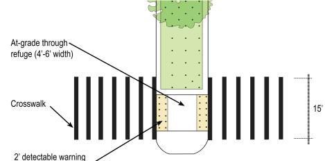
at refuge min. 2' clear waiting area Note: width of median and tactile warning surface to be determined by final engineering drawings
