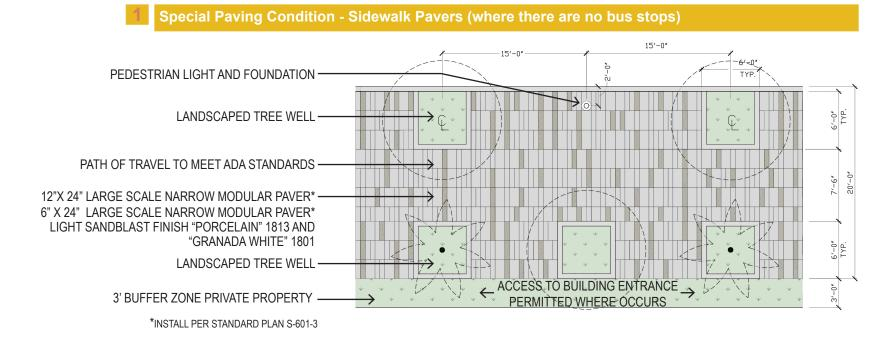
FIGURE 7. Sidewalk Paving Patterns - Special Paving Conditions
