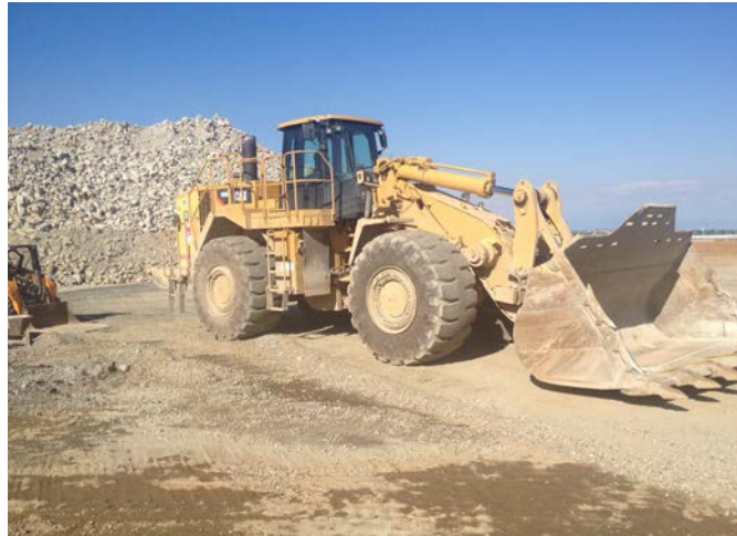
CAT 988H Loader with Tier 4-interim engine used at the concrete crusher at the MSC Project
