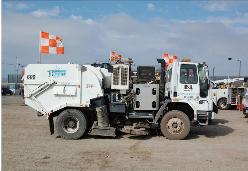
Figure 6-7: PM-10 Compliant Sweeper
