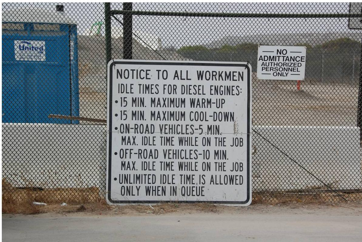
*Figure 6-1: Idle Restriction Signs are Posted Adjacent to Construction Site Entrances*
