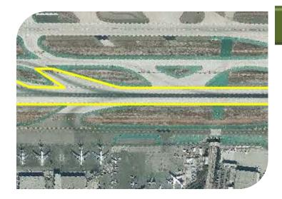
This project will provide improvements to the west end of Runway 25L and temporary runway and taxiway pavement repairs. Additionally, there are improvements to Taxilane C1 which include a Remain-Over-Night (RON) Aircraft Parking Apron and selective grading at the west end of Runway 7L.
