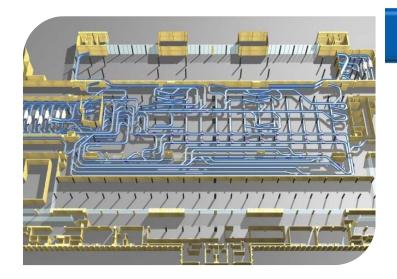
This project enhances and modifies the existing TBIT In-line Baggage Handling System (BHS) to provide better processing and increased throughput of baggage to accommodate future predicted growth. This will be accomplished primarily by revamping the existing layout to provide more BHS Checked Baggage Inspection room.
