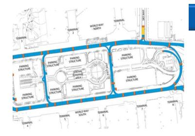
This project provides for the repair and replacement of aging structural expansion joints on the Second-Level Roadway (SLR) in the Central Terminal Area (CTA). An expansion joint is an assembly designed to safely absorb the heat-induced expansion and contraction of adjoining concrete slabs. Specifically, this project will replace and repair joints and deck frames as recommended in the Caltrans bridge inspection report.
