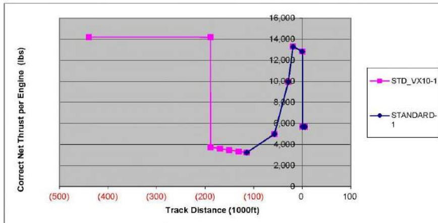
Figure 12 Thrust vs. Distance for 747400 Arrival Standard and Proposed Extended Profile with 10,000 ft. MSL Level Flight Segment
