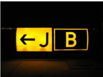
**Direction Signs** have a yellow background with black inscriptions and always include arrows. Direction Signs indicate the name and direction of the taxiway(s) an operator is approaching. Direction signs are often co-located with location signs.
