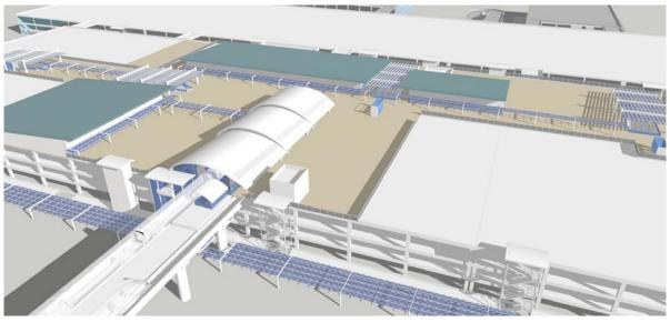
Roof Level layout illustrating CSB, updated south cores, egress stairs, parking and screen walls
