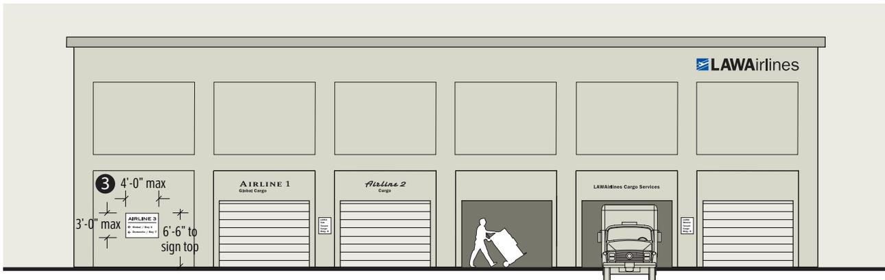
Figure 6e: Directional signs attached to tenant buildings are acceptable but not preferred.
