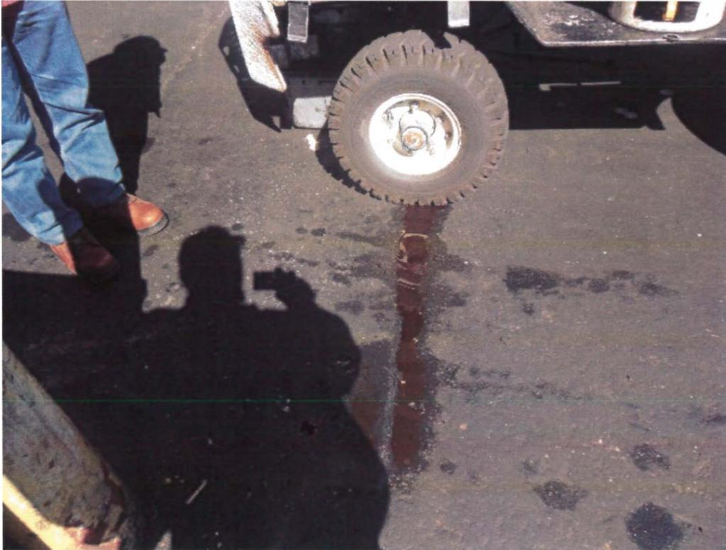
**Photo 1:** Oil spills observed outdoors without BMPs.
