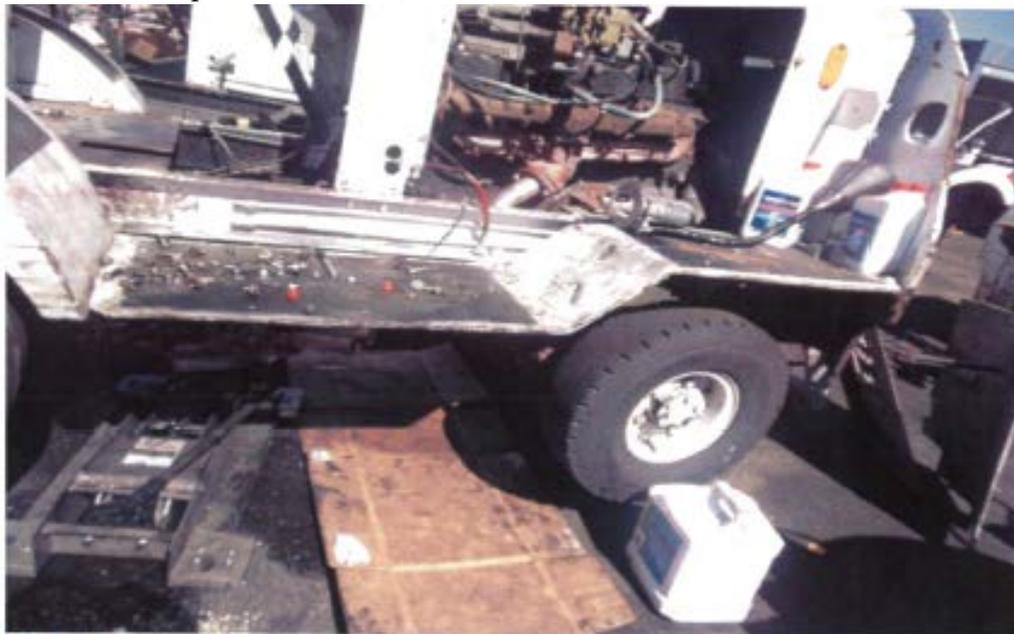
**Photo 17:** Poor housekeeping and poor management practices were observed here. Oily equipment was observed stored outdoors without containment or cover. Oil spills were observed on the ground.
