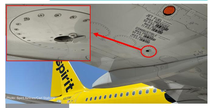
IMAGE: A VORTEX GENERATOR INSTALLED ON AN A320 TO REDUCE NOISE DURING LANDING. **Noise Reduction Efforts** – implementing any equipment, technology, or procedural type effort to reduce aircraft noise; (e.g. retrofitting older A320 aircraft with vortex generators).
