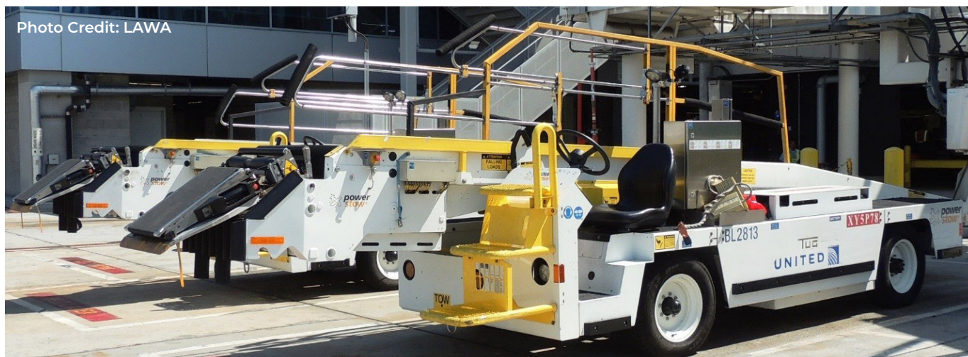
Electric baggage loaders and electric tug at LAX eliminates conventional fuel consumption and reduces air pollution
