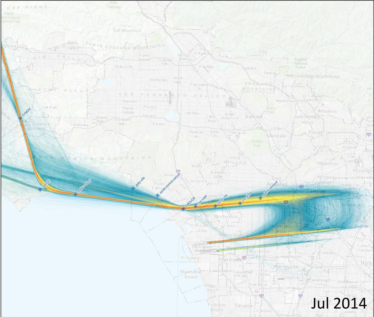
Radar Track Density (8,572 Radar Tracks)
