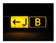
**Direction Signs** have a yellow background with black inscriptions and always include arrows. Direction Signs indicate the name and direction of the taxiway(s) an operator is approaching. Direction signs are often colocated with location signs.
