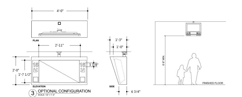
3'-4 1/2" MOUNTING BRACKET 7 8 2'-10 1/2" CEILING 78 BRUSHED STAINLESS STEEL BRACKET COVER STAINLESS STEEL SHROUD INTERNAL FRAMING 3 DATA AND POWER FEED 8 MONITOR BRACKET 2 MONITOR 2 MASKED AND PAINTED FIELD P1 CABINET 3 VINYL GRAPHICS RED/GREEN LIGHTS 6 5 1/2" RED / GREEN LIGHT 6 1'-2 3/8"
