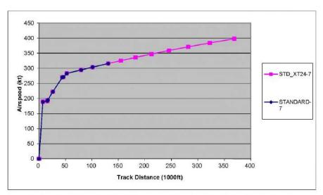
Figure~8~Air speed~vs.~Distance~for~747400~Stage~length~7~Departure, Standard~vs.~Modified~profiles
