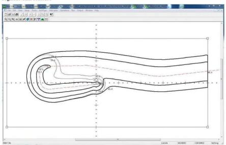
Table 6 compares the noise modeling results for a 777300 arrival using a Standard Arrival profile (from 6,000 ft. AFE) and an extended arrival profile. The extended profile begins in level flight at 10,000 ft. MSL and then descends to the airport runway. Under the flight path, Grid points under the flight path were modeled every 0.5 nm from 50 nm to landing on the runway.
