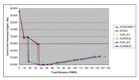
Figure 3 Thrust versus Distance for 777300 Stage Length 7 and Proposed Maximum Weight Profiles
