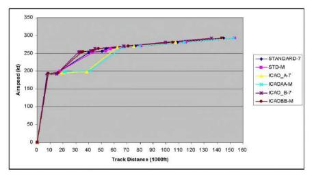
Figure 2 Airspeed versus Distance for 777300 Stage Length 7 and Proposed Maximum Weight Profiles
