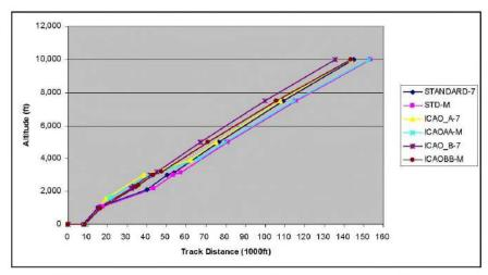
Figure 1 Altitude versus Distance for 777300 Stage Length 7 and Proposed Maximum Weight Profiles
