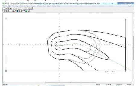
Table 5 compares the noise modeling results for a 747400 arrival using a STANDARD arrival profile (from 6,000 ft. AFE) and an extended arrival profile. The extended profile begins in level flight at 10,000 ft. MSL and then descends to the airport runway. Grid points under the flight path were modeled every 0.5 nm from 50 nm to landing on the runway.
