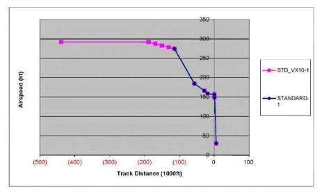
Figure 11 Airspeed vs. Distance for 747400 Arrival Standard and Proposed Extended Profile with 10,000 ft. MSL Level Flight Segment
