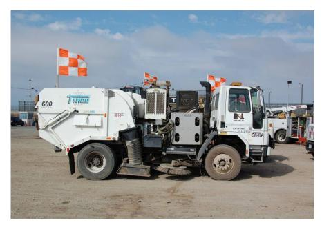
Figure 6-7: PM-10 Compliant Sweeper
