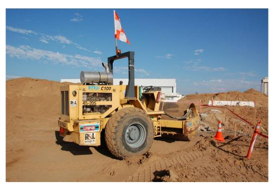
Figure 6 -3: Roller Compactor Equipped with HUSS MK-System VDECS
