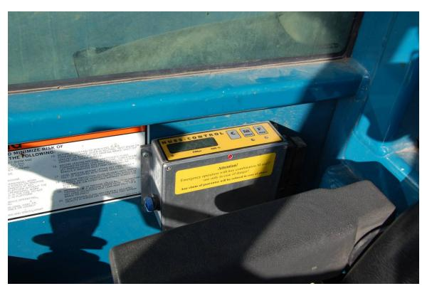
Figure 6-4: VDECS Onboard Monitoring & Driver Notification System
