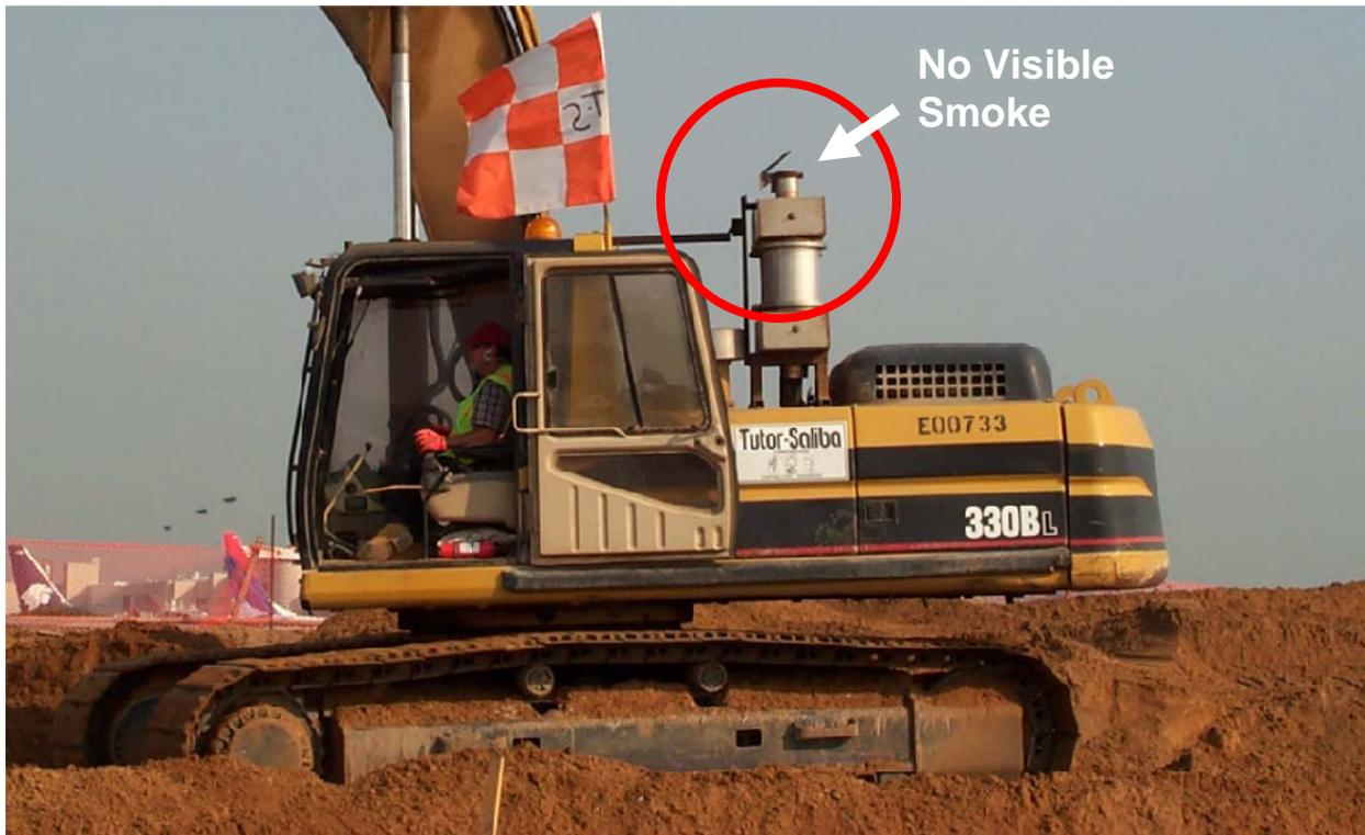
*Figure 6.-13: Caterpillar Excavator with Functioning VDECS*
