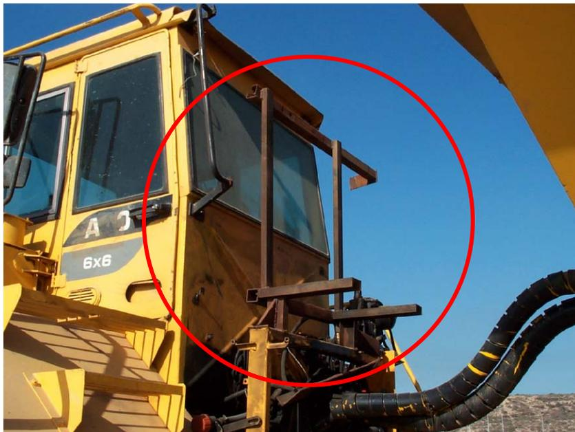
*Figure 2-1: ECS Purifilter VDECS Removed for Maintenance*
