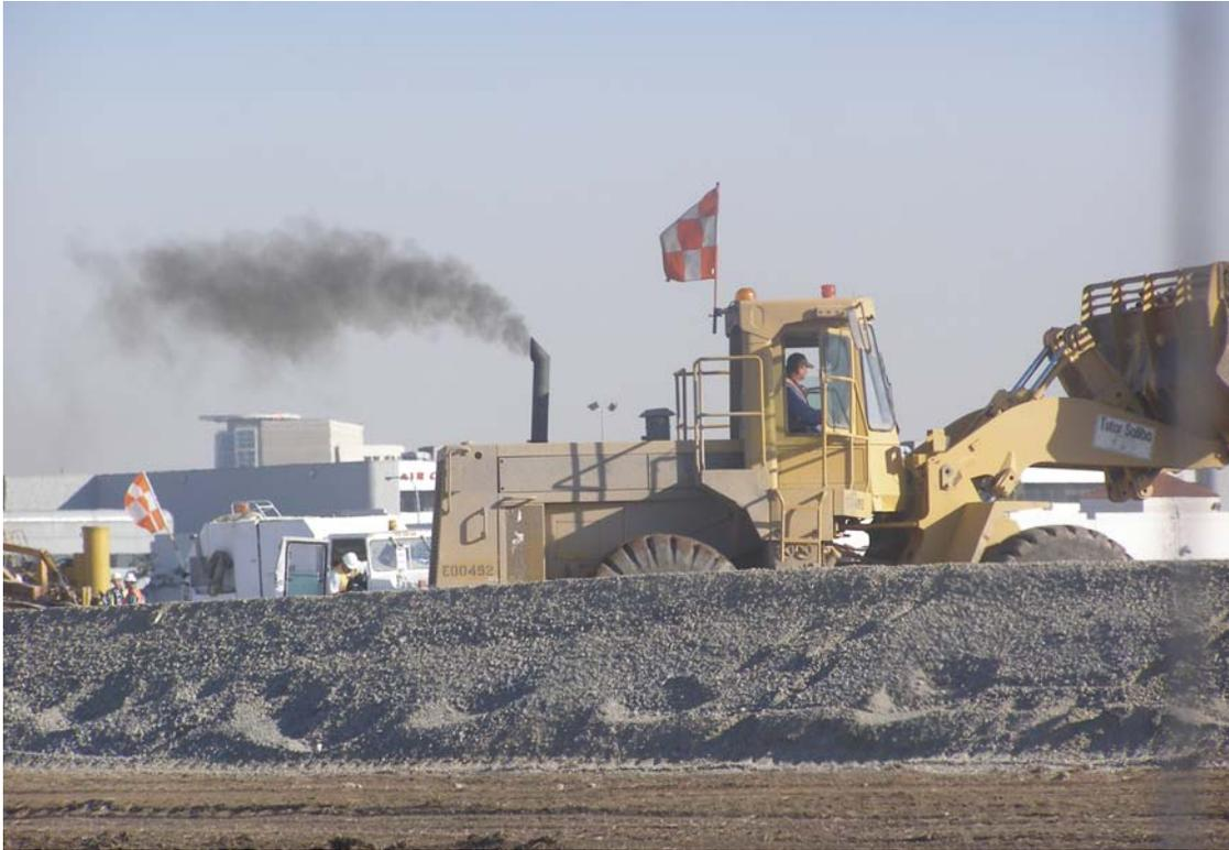
*Figure 6-4: Caterpillar Loader E00492 Emitting High Levels of Exhaust Soot*
