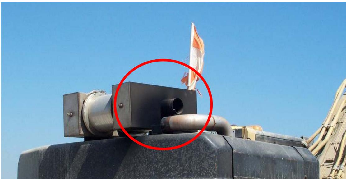
*Figure 6-9: E00732 Was Found to have VDECS Not Hooked Up*
