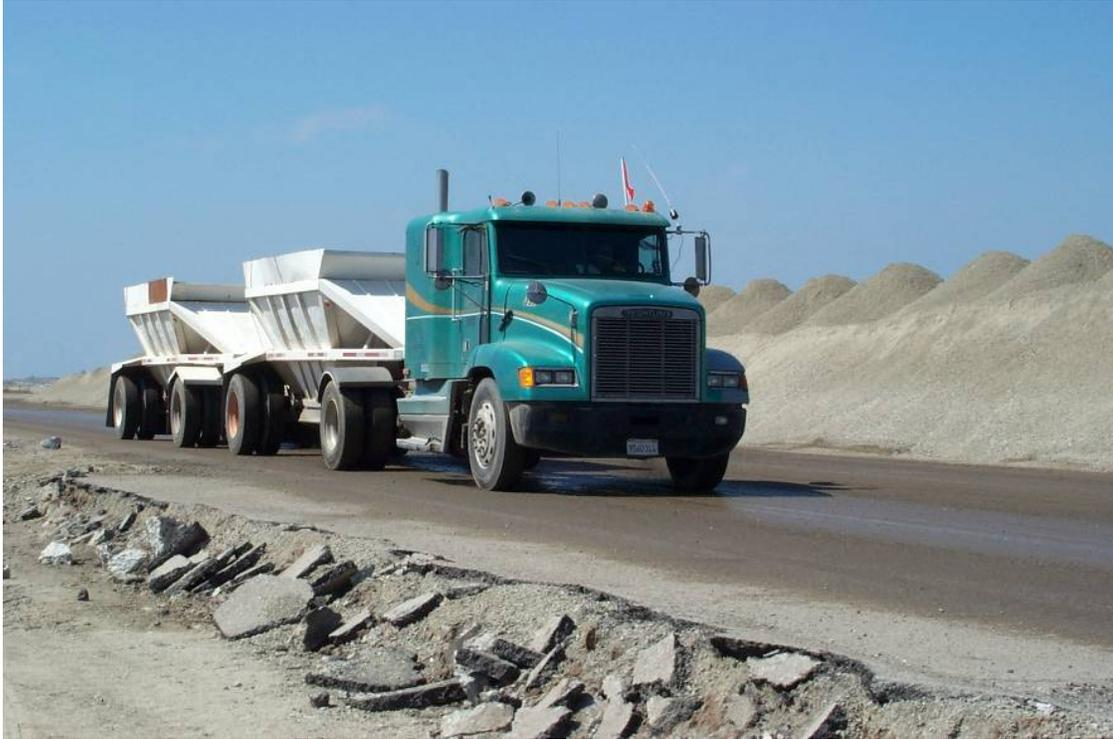
*Figure 6-15: Vigilant Watering of Haul Roads Reduces Fugitive Dust Emissions*
