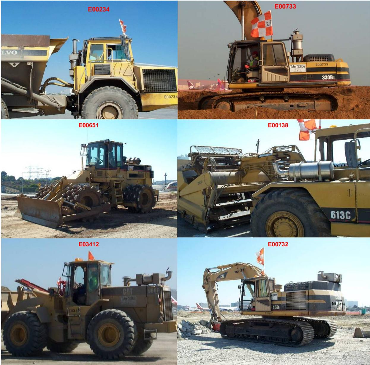
*Figure 1.2-4: Examples of Diesel Equipment Retrofitted with ECS Purifier Device*
