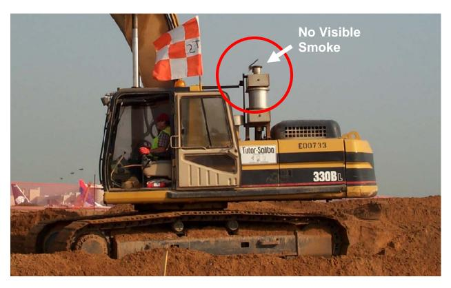
Figure 6.-5: Caterpillar Excavator with Functioning VDECS
