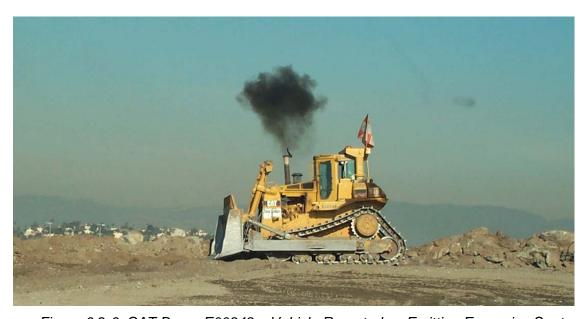
Figure 6.2-6: CAT Dozer E00349 - Vehicle Reported as Emitting Excessive Soot
