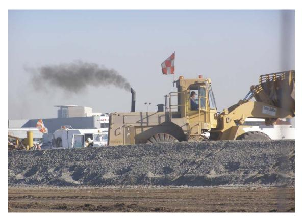
Figure 6.2-3: Caterpillar Loader E00492 Emitting High Levels of Exhaust Soot
