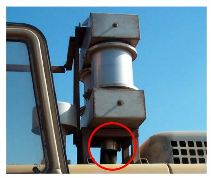
Figure 2-2: Stainless Steel Clamps Replace Welded Exhaust Installation Method
