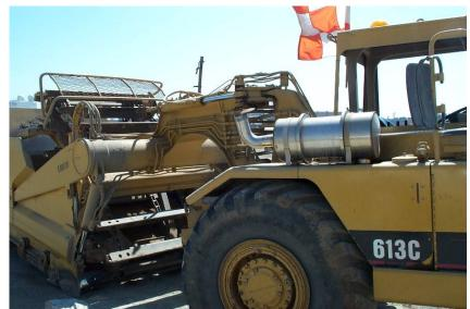
Figure 1.2-5: Caterpillar Scraper E00138 Outfitted with ECS Purifilter
