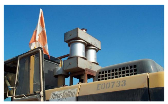
Figure 6-4: E00733 Was Found to have VDECS Sensors Not Hooked Up
