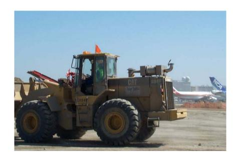
Figure 1.2-6: Caterpillar Loader E03412 Outfitted with ECS Purifilter VDECS
