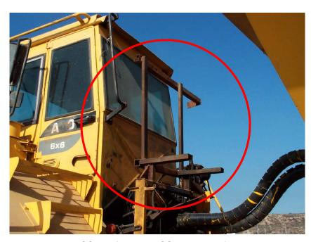
Figure 2-1: ECS Purifilter VDECS Removed for Maintenance
