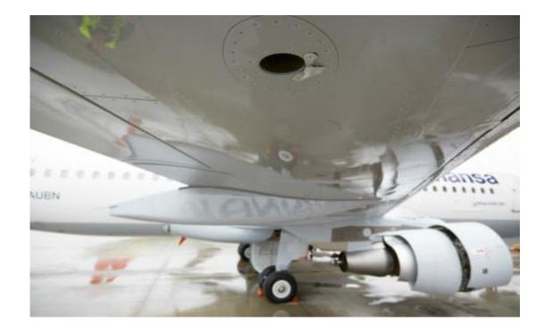
A tiny device, shown here mounted upstream of a circular opening used to equalize the pressure in wing fuel tanks, reduces the whistling noise produced by the Airbus 320. [Photo courtesy of Lufthansa]
