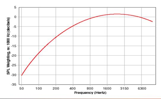
Consistent with EPA's recommendation, the A-weighted level is used by federal, state, and local agencies for environmental noise analyses
