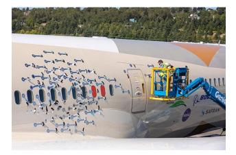
*Figure 1. Microphones attached to the 787-10 Dreamliner ecoDemonstrator*
