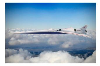
Figure 2. NASA's X-59 Quiet SuperSonic Technology X-plane
