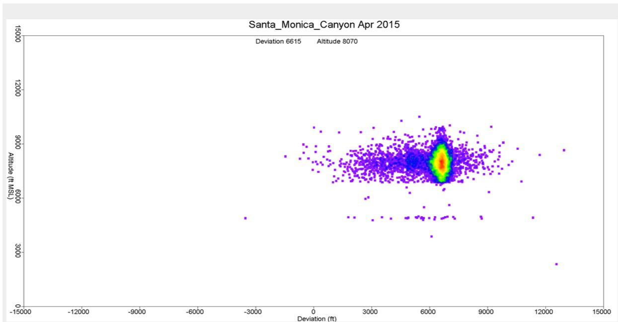
As demonstrated in Figure 30 and Figure 31 above, there was little change in altitude or lateral flight track dispersion west of the SMO VOR/DME during the period from June 2014 to June 2015 over the gate positioned at Santa Monica Canyon. This indicates aircraft throughout this period were flying with consistent frequency over the same general area.
