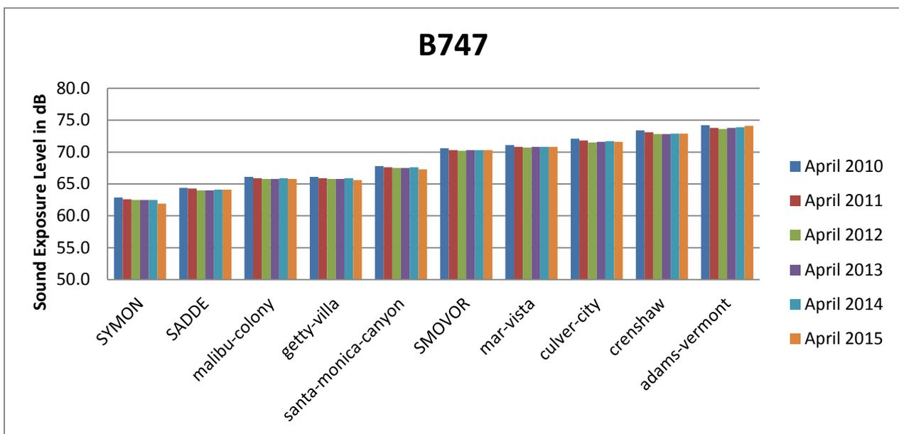
As shown above, the Average Daily SEL values for the Boeing 747 aircraft type changed very little over the six-year period, while the Airbus A380 aircraft type increased in noise level by as much as 4 dB at some of the analysis gates. We did note that the A380 SEL values prior to 2012 were based on very few operations of this newer aircraft type. Therefore, as these aircraft increased operations, the higher
