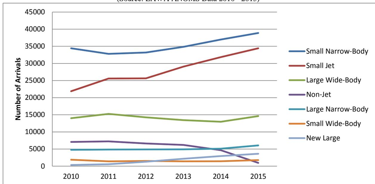
Figures 10 and 11 below provide an alternative representation of the change in aircraft fleet mix from 2010 to 2015 through providing the percentage of aircraft arrivals by aircraft category type for 2010 and 2015 respectively.
