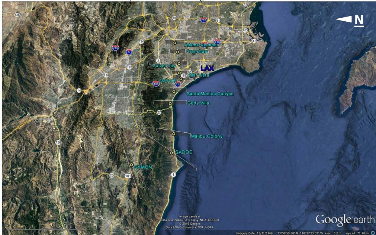
Radar flight track data and gates over analysis locations were used to isolate west and northwest arrivals for this evaluation. Only radar flight tracks that passed through both the "SADDE" and "SMO VOR" gates were included in analysis since nearly all northerly arrivals pass through these two locations. Arrivals approaching LAX from other directions and all departures were excluded from the study.
