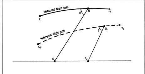
Figure A36-6. Profile characteristics influencing sound level
