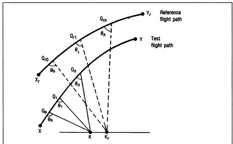
Figure A36-10. Correspondence between measured and reference flight paths for the application of the integrated method of adjustment
