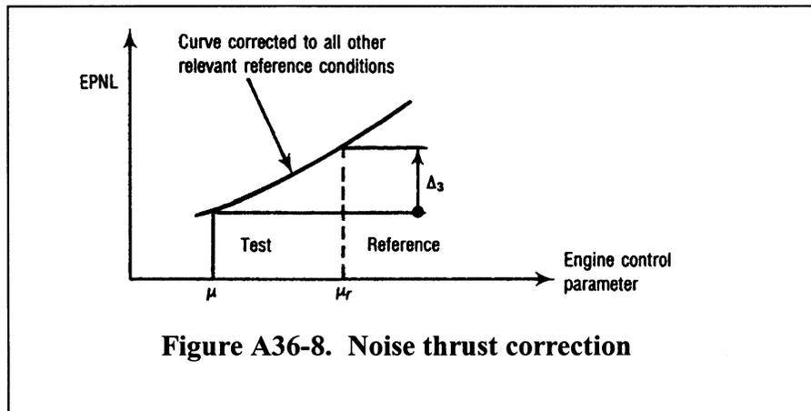
**Figure A36-8. Noise thrust correction**
