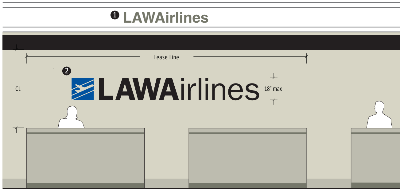
Figure 3c: Dimensional copy is the preferred treatment for corporate signature signs on walls behind ticket counters.
