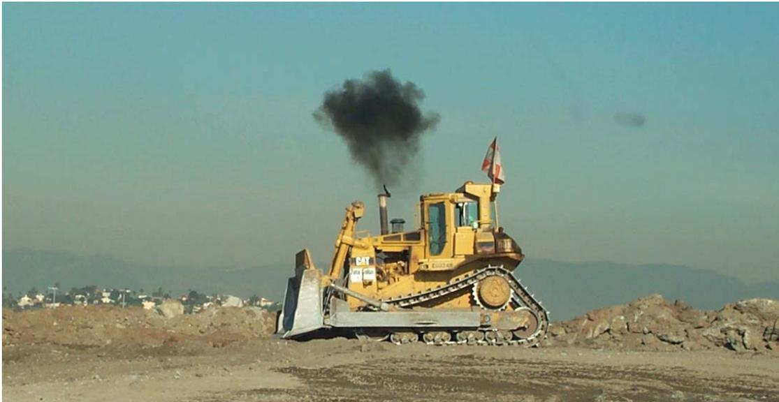
*Figure 6 -7: CAT Dozer E00349 – Vehicle Reported as Emitting Excessive Soot*
