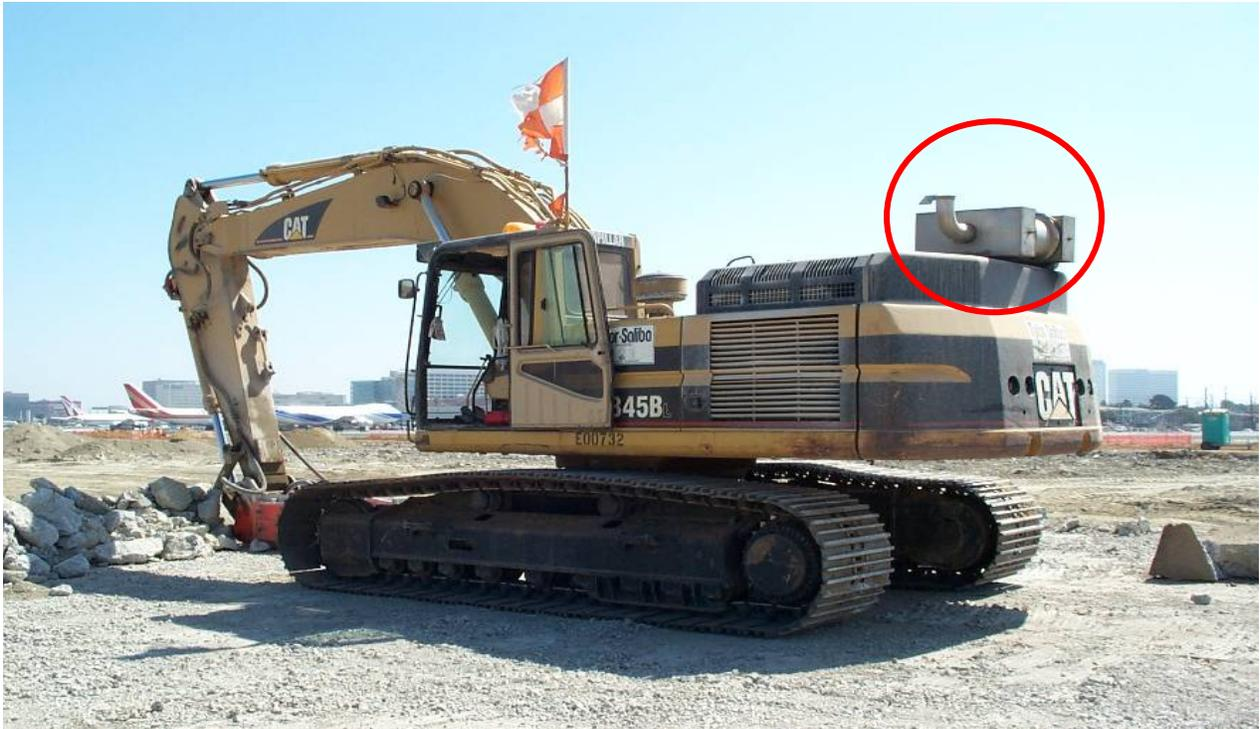
*Figure 6-8: Caterpillar Excavator E00732 Equipped with ECS Purifilter VDECS*
