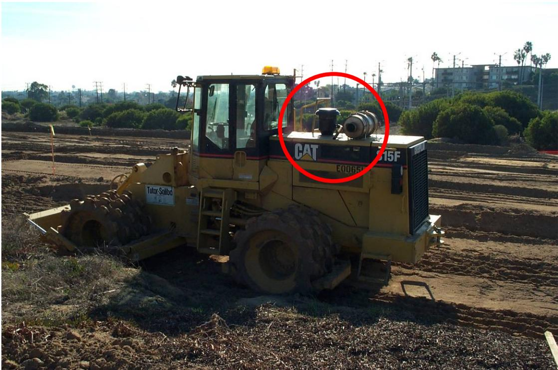
Figure 6-11: CAT Compactor E00651 is Equipped with an ESC Purifier VDECS
